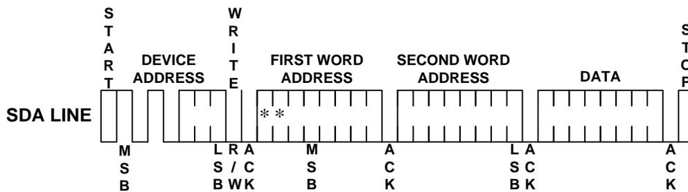
Figure 3: Byte Write
