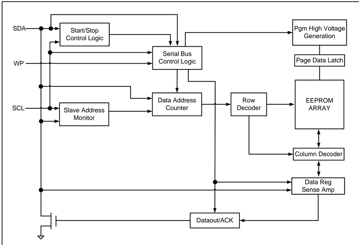
Figure 2: Block Diagram
