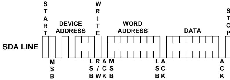
Figure 5: Byte Write
