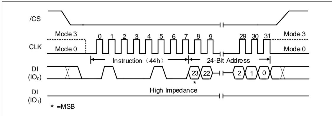
Figure 35. Erase Security Registers Instruction (SPI Mode only)
