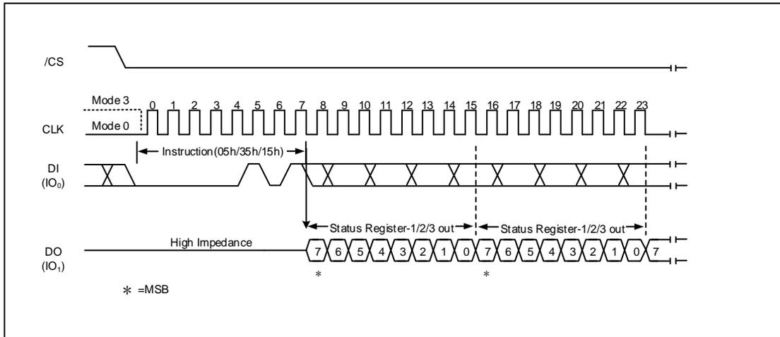
Figure 8a. Read Status Register Instruction (SPI Mode)
