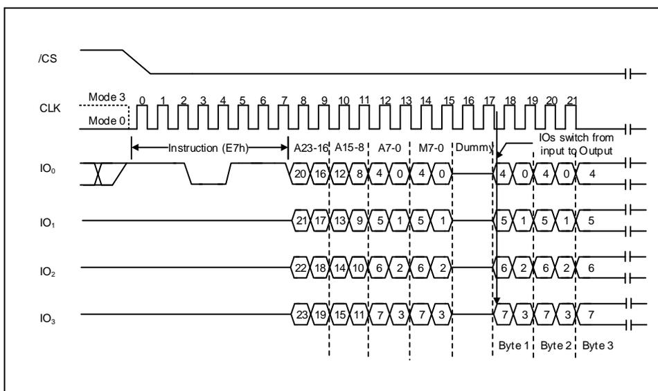
Figure 16a. Word Read Quad I/O Instruction (Initial instruction or previous M5-4 = 10, SPI Mode only)
