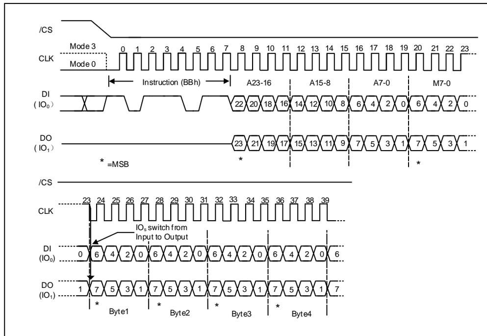
Figure 14a. Fast Read Dual I/O Instruction (Initial instruction or previous M5-4 = 10, SPI Mode only)
