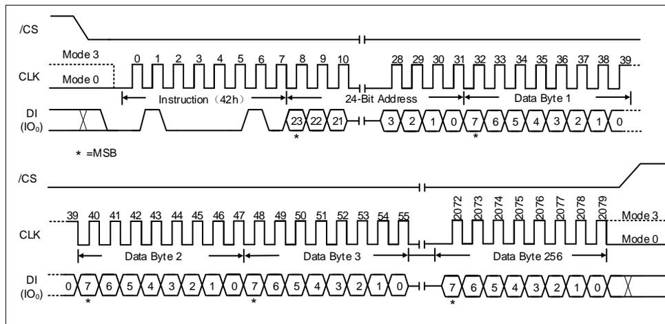
Figure 36. Program Security Registers Instruction (SPI Mode only)
