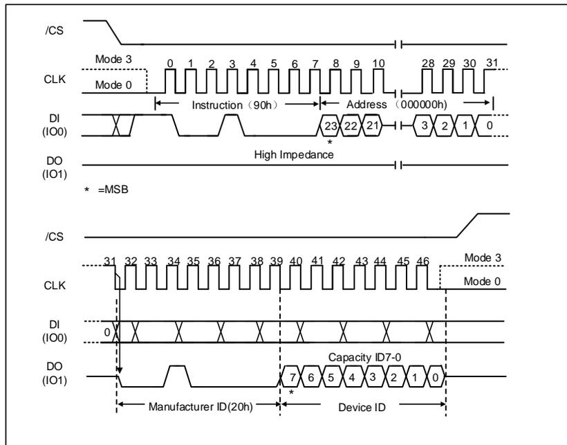
Figure 29. Read Manufacturer / Device ID Instruction (SPI Mode)
