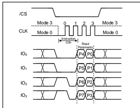
Figure 38. Set Read Parameters Instruction (QPI Mode only)
