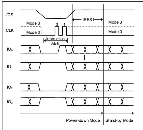
Figure 28b. Release Power-down Instruction (QPI Mode)
