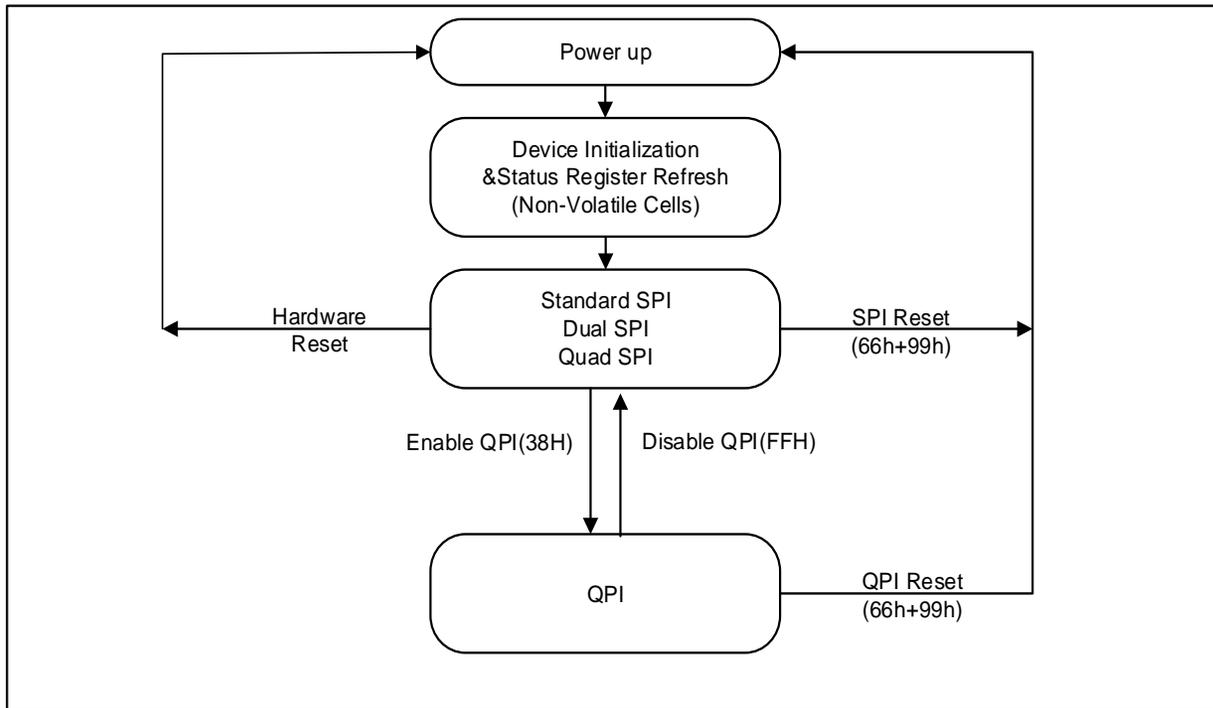
Figure 3. XM25QW128C Serial Flash Memory Operation Diagram
