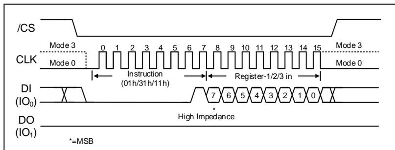
Figure 9a. Write Status Register-1/2/3 Instruction (SPI Mode)
