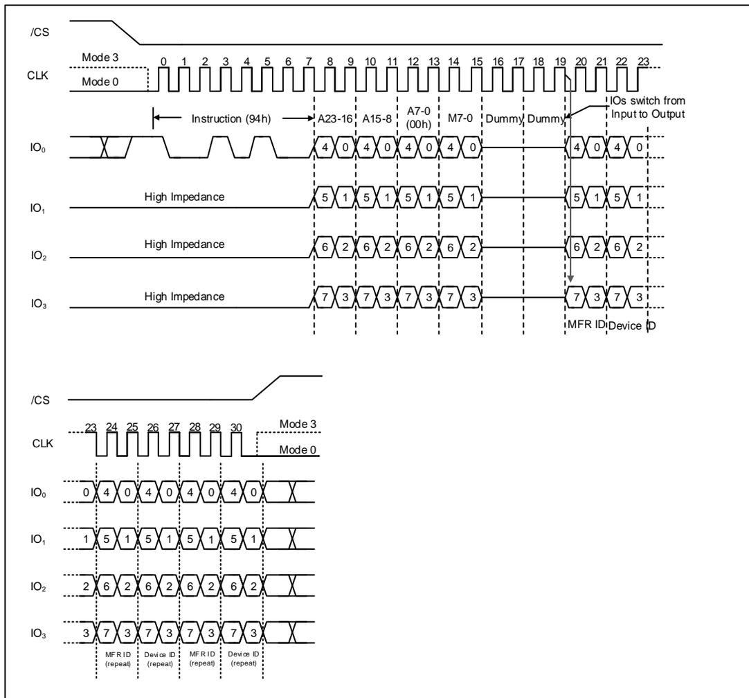
Figure 31. Read Manufacturer / Device ID Quad I/O Instruction (SPI Mode only)
