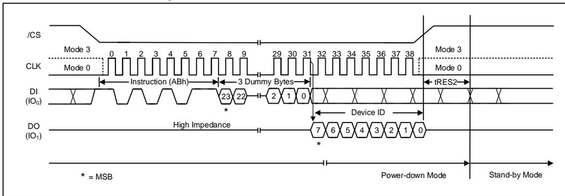
Figure 28c. Release Power-down / Device ID Instruction (SPI Mode)
