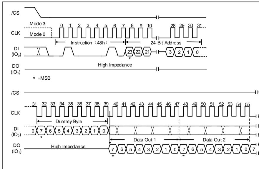
Figure 37. Read Security Registers Instruction (SPI Mode only)
