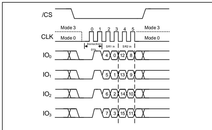
Figure 9d. Write Status Register-1/2 Instruction (QPI Mode)
