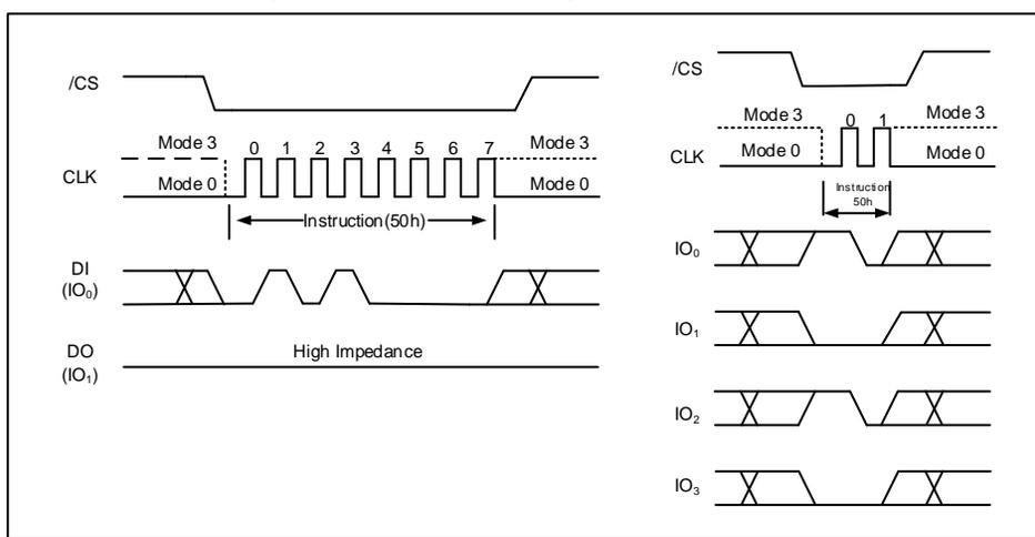
Figure 6. Write Enable for Volatile Status Register Instruction for SPI Mode (left) or QPI Mode (right)
