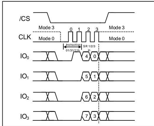
Figure 9b. Write Status Register-1/2/3 Instruction (QPI Mode)
