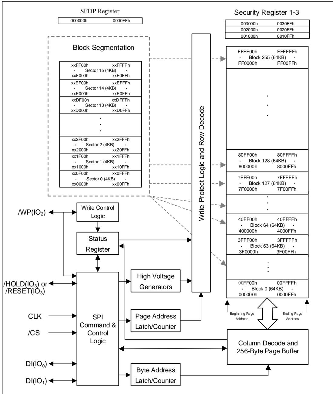
Figure 1. XM25QW128C Serial Flash Memory Block Diagram
