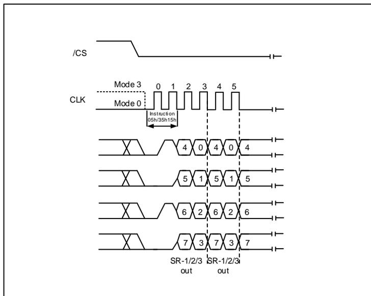
Figure 8b. Read Status Register Instruction (QPI Mode)
